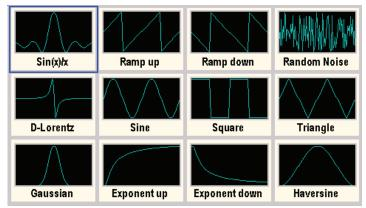
Select from 12 different predefined arbitrary waveforms or store and recall up 13 additional custom waveforms from the internal memory.
