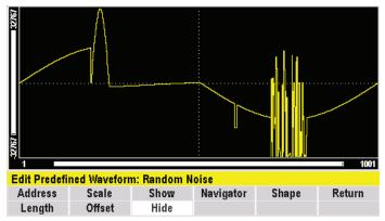
From the front panel, arbitrary waveforms can be defined from scratch by entering data point-by-point or by loading and modifying predefined waveforms.
