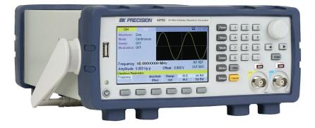
The 4078C Series Arbitrary/Function Waveform Generators are versatile, high-performance dual-channel arbitrary waveform generators with 16-bit amplitude resolution. They provide variable output voltages from 0 to 10 Vp-p into 50 ohms, up to 20 Vp-p into an open circuit, and a continuously variable DC offset to bias the output signal at a desired level.
