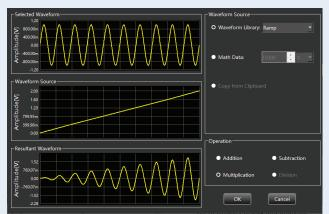
Generate complex arbitrary waveforms with tools that allow you to draw, edit, and combine waveforms.
