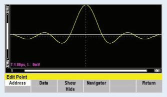
Create or edit arbitrary waveforms directly from the front panel by defining individual points, lines, or copying and pasting sections.
