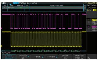
Serial bus decoding supports  $I^2C$ , SPI, UART, CAN and LIN protocols. Information can be quickly displayed in a tabular format.
