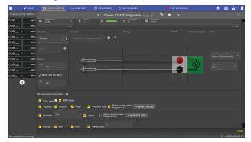
The channel configuration menu offers an intuitive design to ease measurement setup. Additionally, users can record True RMS, frequency, counter, PWM, derivative, integral average, min, max, and peak to peak measurements without the need to use another physical channel.
