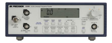
The 1820B Series Universal Frequency Counters are portable, battery-operated, universal counters with a 0.5" 10-digit liquid crystal display (LCD). These instruments measure a wide frequency range from 0.001 Hz to 6 GHz (1826B) and include measurement functions for frequency, period, ratio, pulse width, and count.
