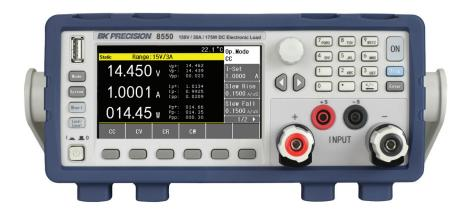
The 8550 Series DC electronic loads provide many features and capabilities typically found in performance instruments, at a value price. Capable of sinking 350 W in a compact benchtop form factor, this series is well equipped for testing and evaluating power supplies, DC-DC converters, batteries, battery chargers, and photovoltaic arrays.
