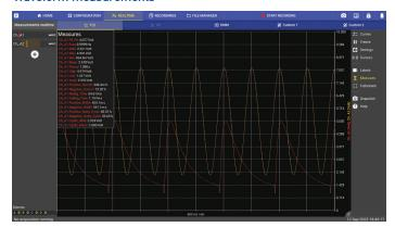
Automatically calculate up to 19 different waveform measurements including, amplitude, RMS, mean, frequency, rise time, and fall time.
