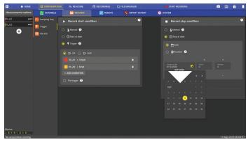
Configure the trigger settings to start and stop acquisition manually, at a specified time, or through a combination of one or multiple channel(s).
