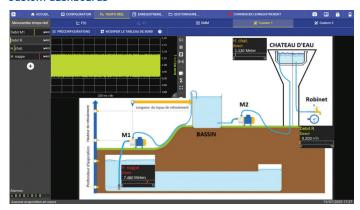
Measure and visualize data as real-time waveforms and numeric values on a customizable dashboard. Import circuit diagrams or system images to display on the dashboard.
