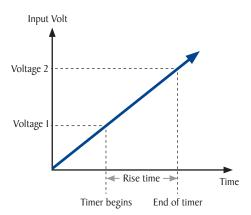
The resulting rise/fall time measurement is displayed on screen with 0.1 s resolution.
