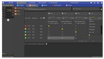
Record data at up to 4 different user configurable sample rates simultaneously. Allocate channels to slower rates or higher rates on a per channel basis for efficient use of hard drive space.
