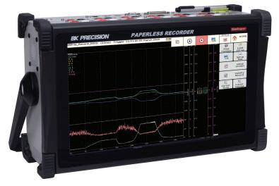
The DAS1700 high speed, configurable data acquisition system combines a fast sampling rate, deep memory, and a large touch screen display. The system also includes built-in software tools for power analysis and a mathematical function editor for performing calculations between multiple channels.
