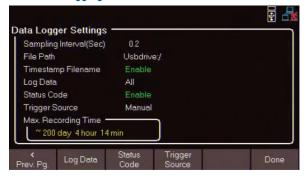
Log voltage, current, or both at a user-defined sampling interval adjustable from 0.2 seconds to 5 minutes directly to an external USB flash drive. Data points are saved as a CSV file with date and time stamp.
