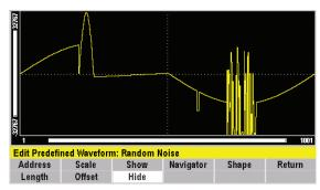
Draw lines, and modify waveforms on a point-by-point basis, or combine aspects from multiple predefined waveforms such as injecting noise into a sine wave.
