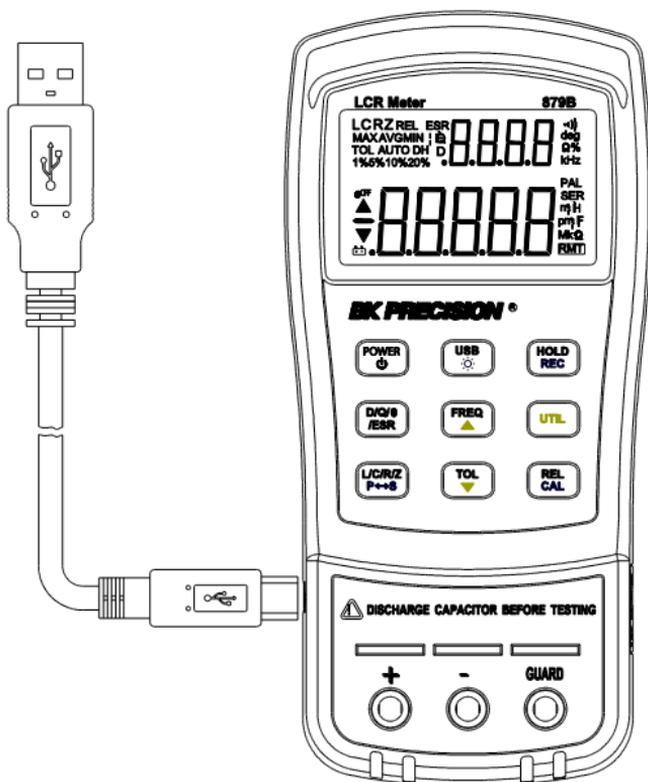
Figure 14 – Connexion USB
