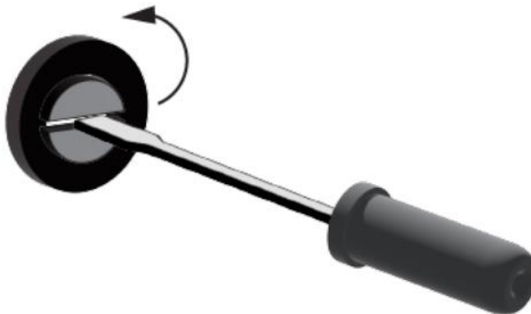
Figure 2.1 Extraction du fusible
