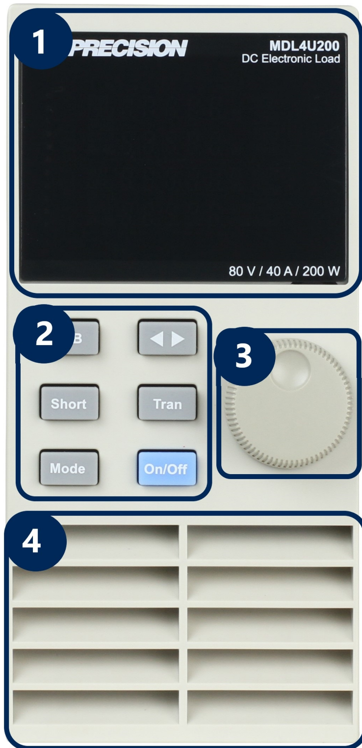
Figure 6.7 Module Front Panel
