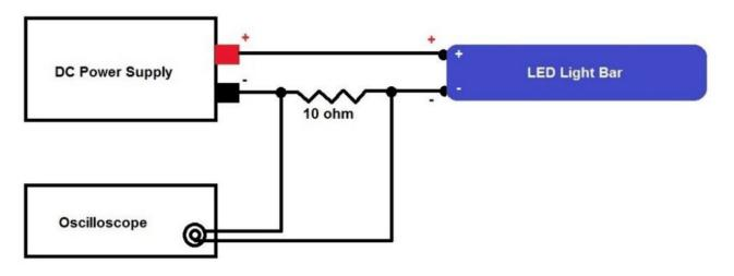
Figure 4.1 LED Testing Example
