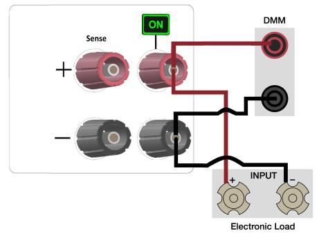
Figure 12.1Front Panel Wiring Diagram
