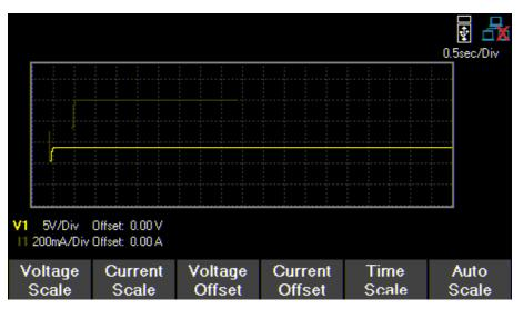
Figure 3.4Live Output Monitoring Display
