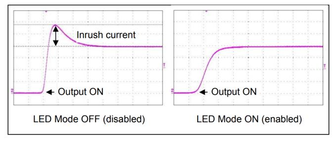
Figure 4.2 Inrush Current With and Without LED Mode Enabled
