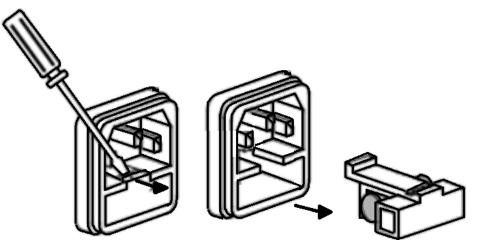
Figure 2.1 Fuse Removal
