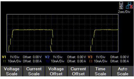
Figure 3.5 Live Output Monitoring Display
