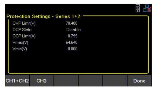
Figure 4.14 Parallel CH 1+2 Protection Settings
