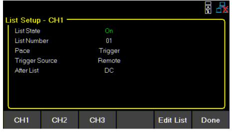
Use the softkeys to select one of the channels CH1, CH2, or CH3.
