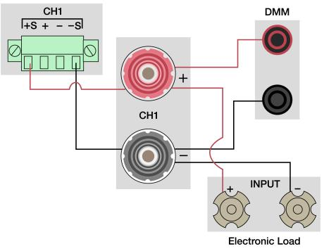
Figure 11.1Front Panel Wiring Diagram
