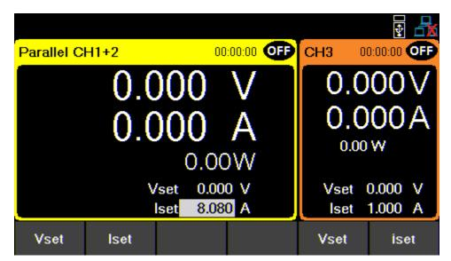
Figure 4.12 Parallel CH 1+2 Main Display 9141
