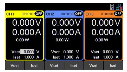
Figure 3.3 Three Channel Display
