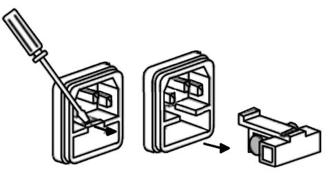
Figure 2.1 Fuse Removal
