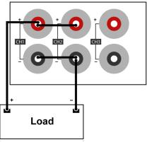
Figure 14 - Parallel Wiring Mode, CH1+CH2
