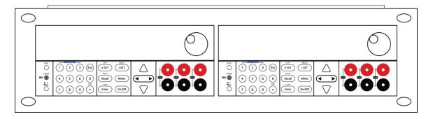
To rackmount two instruments side-by-side, order rackmount kit IT-E151, the front cover panel is not needed.
