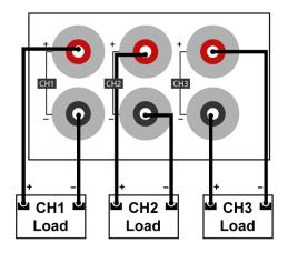
Figure 11 - OFF (normal) Wiring Mode
