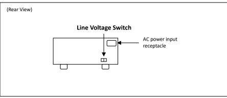
Figure 6 - Model 9129B Line Voltage Switch Location
