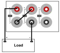
Figure 12 - Series Wiring
