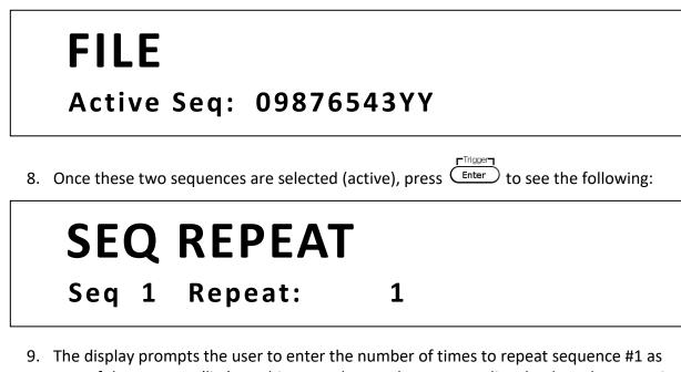
9. The display prompts the user to enter the number of times to repeat sequence #1 as part of the program (list). In this example, use the current adjust knob or the numeric keypad to enter 2. Press inter and the same prompt will immediately follow for sequence #2. Enter 3 and then press inter.
