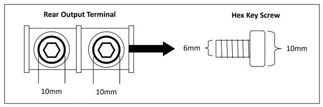
Figure 2.3 - Rear Output Terminal
