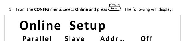
2. While **Parallel** or **Series** is flashing, use ▲ ♥ keys to toggle between the two options. Set to **Parallel** for parallel connection and **Series** for series connection.
