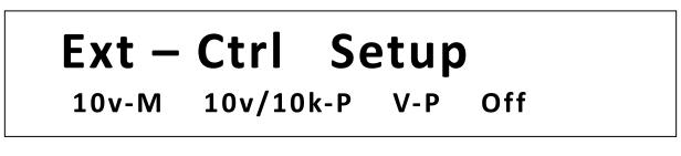
2. Select the third item V-P or R-P so that it is blinking. Use the ▲ ♥ keys to change between V-P or R-P.
