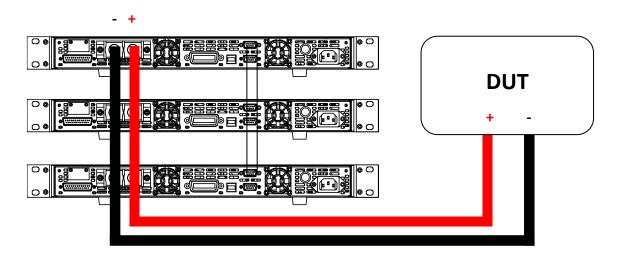
Figure 3.4 – Master/Slave Parallel Connection Diagram
