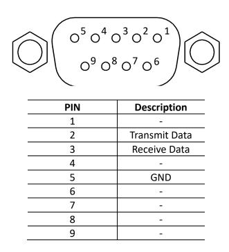
A straight pin-to-pin DB9 female to DB9 male serial cable is required for using the RS-232 interface. Do not use a null modem or crossover DB9 serial cable.
