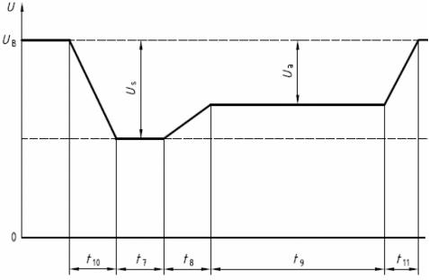
Figure 3.8 – Test Pulse waveform (DIN 40839)
