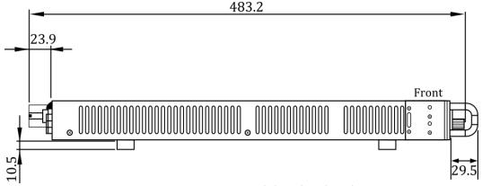
Figure 1.2 – Side View for 9115/B/9115/B-AT/9116/B
