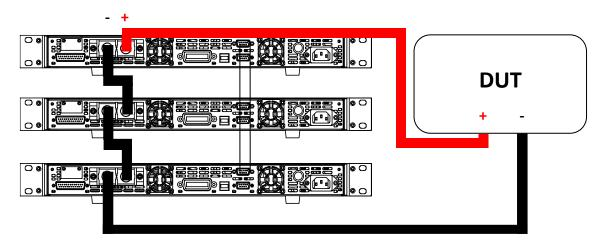
Figure 3.5 - Master/Slave Series Connection Diagram
