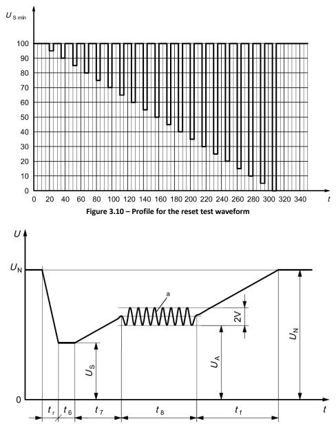
Figure 3.11 – Starting profile waveform
