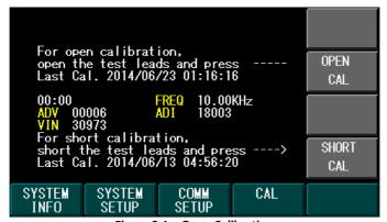
Figure 3.1 - Open Calibration
