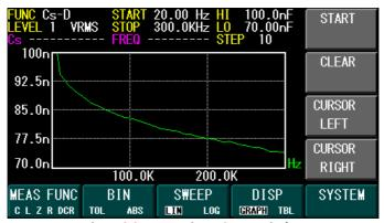
Figure 3.31 - Post Linear Sweep Display
