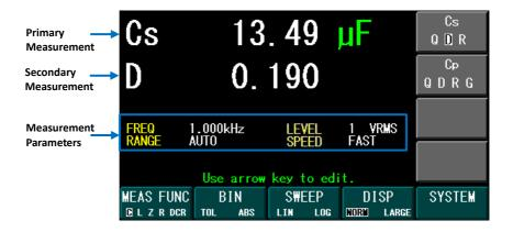
Figure 3.10 - Measurement Function Display
