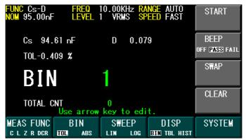
Figure 3.23 - - Bin Mode View (Tolerance Mode)
