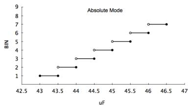
Figure 3.16 - Bin Setup Absolute Mode Graph
