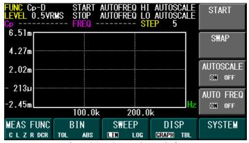
Figure 3.27 - Sweep Linear Display
