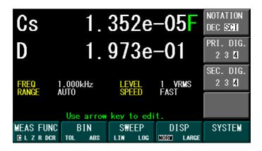
Figure 3.13 - Display Function (Notation)
