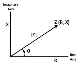
Figure 3.6 - Complex Impedance Plane
