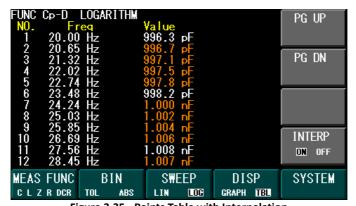
Figure 3.35 - Points Table with Interpolation
