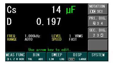
Figure 3.12 – Display Function (Primary and Secondary Digits)
