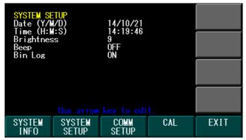
Figure 4.3 - System Setup Screen
