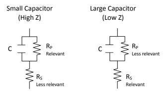
Figure 3.8 - Equivalent Capacitor Circuit
