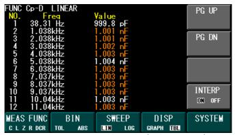
Figure 3.29 - Sweep Table Display (with INTERP ON)
