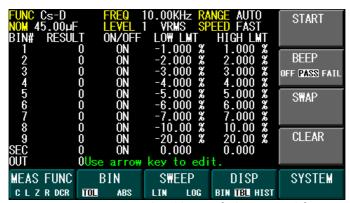
Figure 3.17 – Bin Mode Table View (Tolerance Mode)
