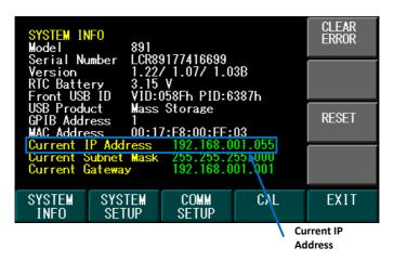
Figure 6.1 – Current IP Address
