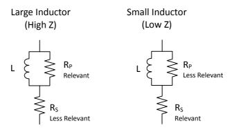
Figure 3.9 - Equivalent Inductor Circuit
