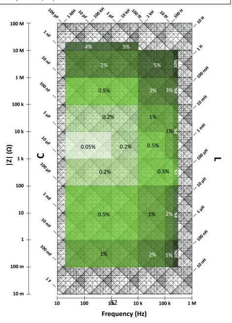
Figure 8.1 - Measurement Accuracy Chart
