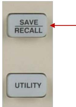
The scope can save 2 groups’ reference waveforms, 20 groups’ setups, and 10 waveforms to the oscilloscope’s internal memory. There is a USB Host interface in the front panel of the oscilloscope where you can save setup data, waveform data, waveform interface image, CSV file to a USB flash drive. Setup data and waveform data can be recalled to the oscilloscope. Picture data and CSV file can’t be recalled to the oscilloscope, but it can be opened on a computer.
