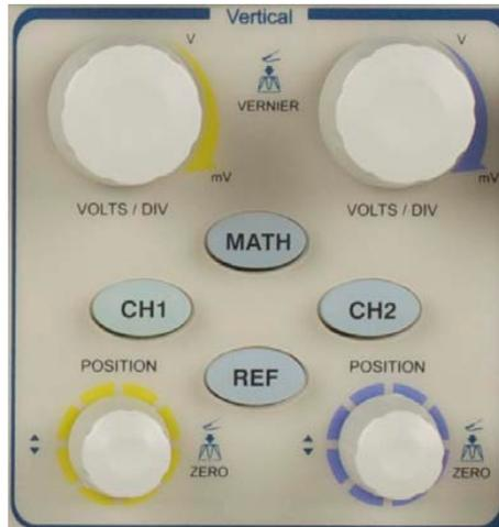
Figure 14 - Vertical System Controls
