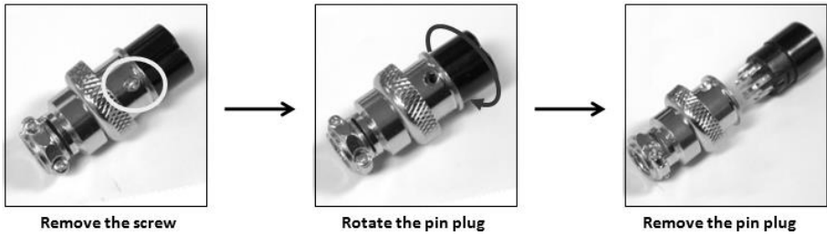
Figure 4 - Remote Control Connector
