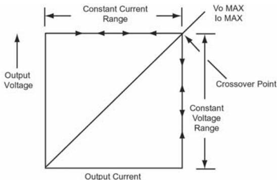
**Figure 4 – CC/CV Characteristic**
