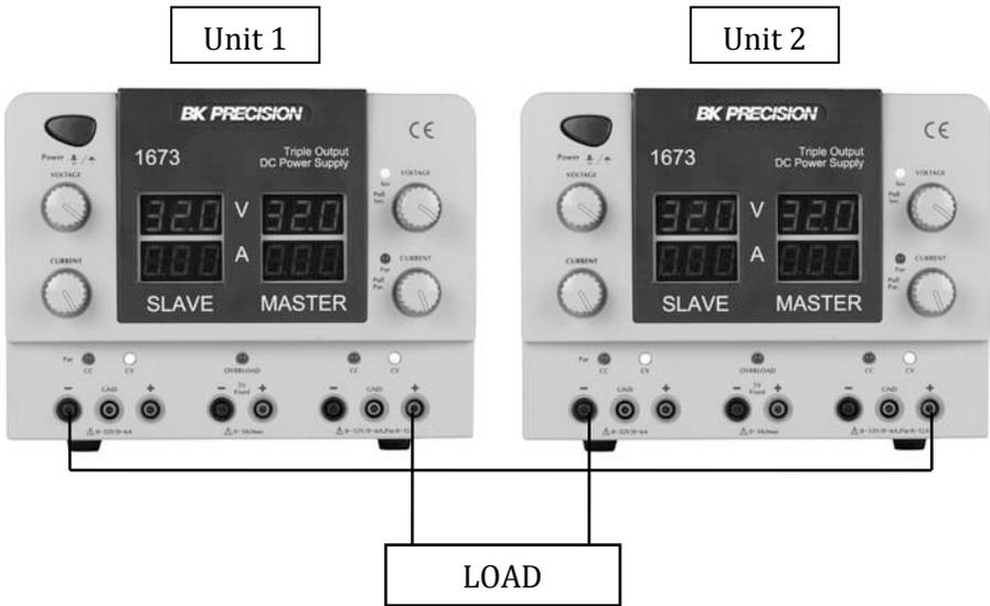
**Figure 7 – Connecting Multiple Units in Series**
