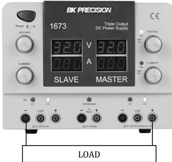
**Figure 5 – Series Tracking Mode Load Connection**
