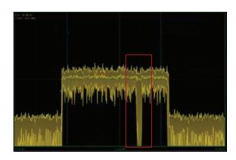
Figure Ib. Identification of a signal dropout with Real-Time Power Processing.
