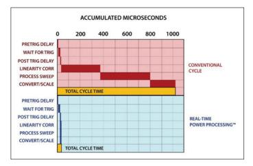
Figure Ia. Comparison between conventional power measurement sample processing and Real-Time Power Processing.
