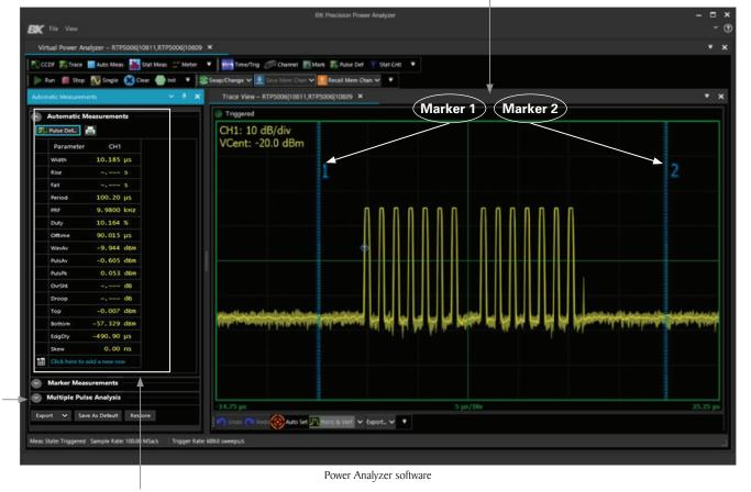
To simplify testing, the RFP3000 Series can automatically measure and calculate 16 common power and timing parameters and display the parameters of interest. Other parameters include: rise time, fall time, pulse average, overshoot, and droop.
