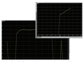
Figure 2b. "Conventional" power meter waveform analysis with 10 ns/div time base and I sample per division.
