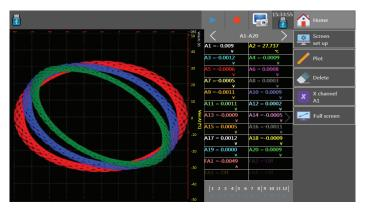
XY mode for plotting one varying voltage versus another
