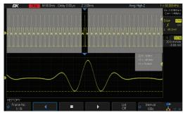
The hardware-based Zoom function used with the record lengths of 140 Mpts enables users to capture more of their signal and quickly zoom into the event of interest.
