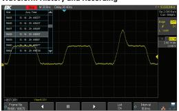
Quickly scroll through millions of points with History Mode's playback functionality to find difficult to capture events. Eliminate unnecessary idle signals and dead-time by selectively capturing up to 80,000 segments.
