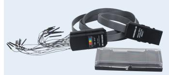
The I6-channel color-coded logic probe consists of two eight-channel pods. To make contact with the DUT, the probe connects directly to square pins or clips to test points using the included grabbers. With an input capacitance of only I8 pF and I00  $k\Omega$  input impedance, the probe protects the integrity of your signal. The probe is included with MSO models.
