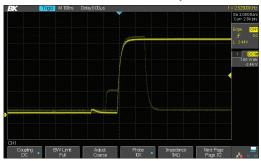
The 140,000 wfms/s update rate in normal mode helps detect infrequent anomalies and glitches.
