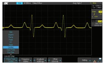
Take advantage of the generator's 10 built-in waveforms or generate up to 4 of your own arbitrary waveforms via waveform editing software.
