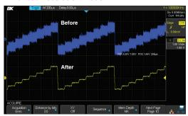
Enhanced Resolution (Eres) mode minimizes signal noise to reveal hidden detail when the signal is difficult to trigger and averaging methods are confined.
