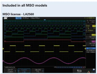
The 16 integrated digital channels are displayed along-side analog channels allowing users to view up to 20 time-correlated channels with shared triggering and acquisition on one screen. The LA2560 license enables the 16 digital channels of the 2560 Series and is included with MSO models.
