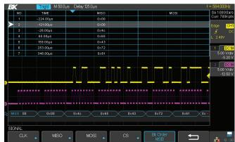
Select up to 2 serial bus protocols I2C, SPI, UART/RS232, CAN, and LIN and decode concurrently from analog and MSO channels. Decode information in real-time and display in binary, decimal, hex, or ASCII.
