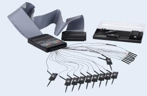
The I6-channel color-coded logic probe consists of two eight-channel pods. To make contact with the DUT, the probe connects directly to square pins or clips to test points using the included grabbers. With an input capacitance of only 8 pF and I00  $k\Omega$  input impedance, the probe protects the integrity of your signal. The probe is included with MSO models.
