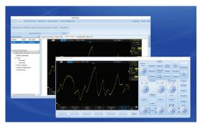
PC software is provided (free download at www.bkprecision.com) for seamless integration between the oscilloscope and PC. Capture and transfer waveforms, screen images, setups and measurement results to a Windows PC via the USB device port on the back of the instrument. A USB host port on the front allows for quick and easy screen saving.
